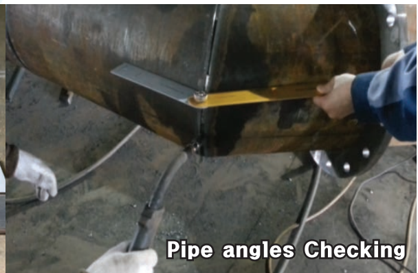
Easy to mark and check angle
