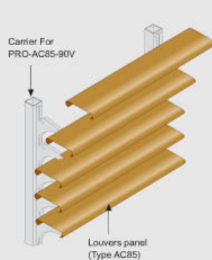
Isometric View: PRO-AC85-90V Vertical Sun Louvers
