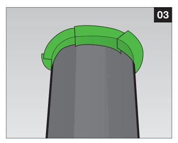
Apply Rissan around circular parts in layers
